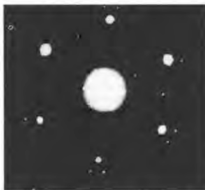
Fig. 4. Electron diffraction from a Cu/Ni superlattice. The absence of rings indicates the single-crystal nature of the sample. The weaker spots surrounding the six main spots are due to the layering.
